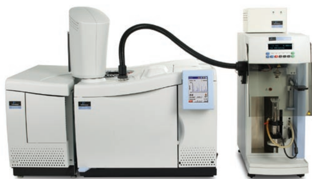
Figure 1. Clarus 600 GC/MS interfaced to the Pyris 1 TGA.
