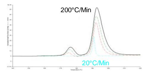
In the case of the above sample of Carbamazepine, the use of the second derivative curve also shows the existence of a third peak on the front edge of the main melting peak. This is shown below
